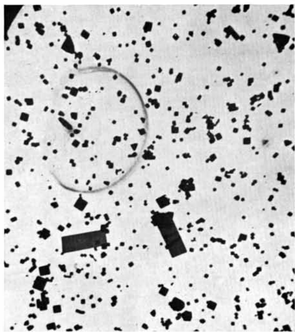
Fig. 1. Shadow micrograph taken in convergent-beam apparatus, showing region of magnesium oxide smoke with cube and plate crystals. Long edge of plates is \sim 1.0 micron.
